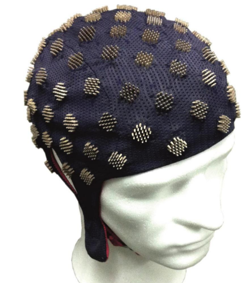
Prototyoe of 97 equidistant multi-pin dry electrode cap.
